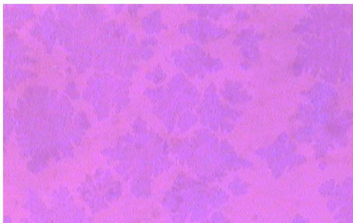
Monolayer graphene flowers grown by CVD on copper and transferred onto silicon dioxide/silicon wafer
